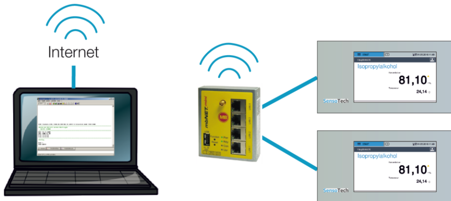
TCP/IP connection (VPN via UMTS/3G router)
